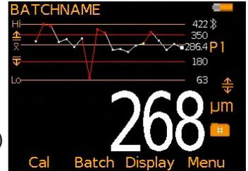
The readings are displayed as white or red points; white if a reading is within limits (or no limits have been set), and red if outside set limits.
