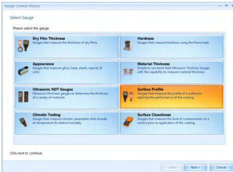
These instructions will inform the user how to download data from an Elcometer 224 surface profile gauge. All appropriate Elcometer gauges can be downloaded in a similar way.
