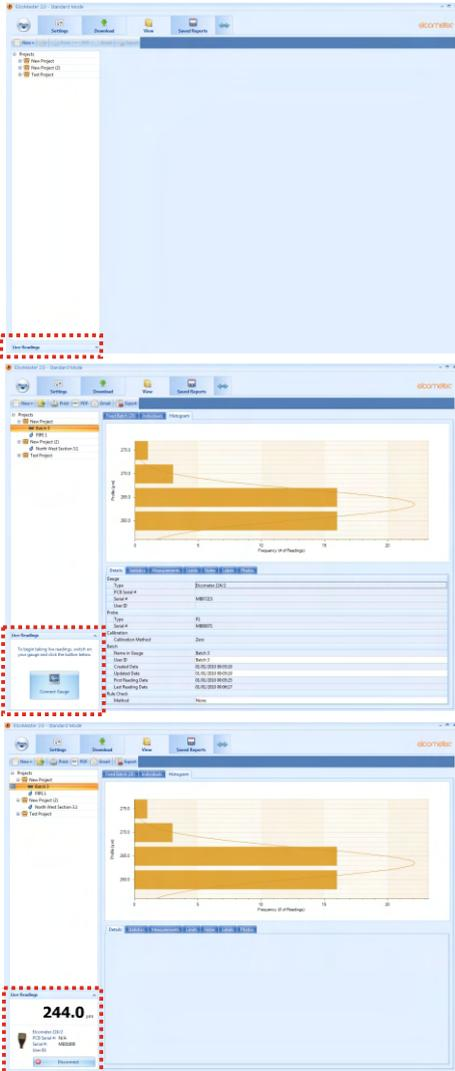
Once the gauge has been connected to ElcoMaster™ 2.0 (see pages 33 - 35), switch on your gauge and click the 'Live Readings' button on the View Action Tab
