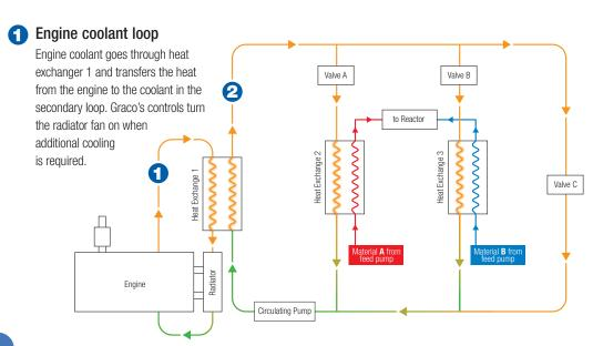
Secondary coolant loop — Coolant in the secondary loop continually circulates when valve C is open, maintaining a consistent temperature. When material heating is required, valve C closes, and valves A and B open. This allows the coolant in the secondary loop to go through heat exchangers 2 and 3, thereby transferring the heat to the A and B materials.
