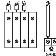
**350-415 V ac, 3-phase Wye:** Use a screwdriver to connect four power leads to the top terminals as shown. Connect neutral only to N. Connect green to ground (GND). See page 18 for proper jumper positions.
