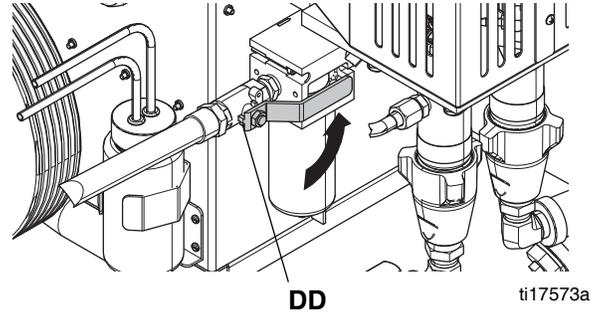
6. Turn the air regulator counterclockwise to 0 pressure.
