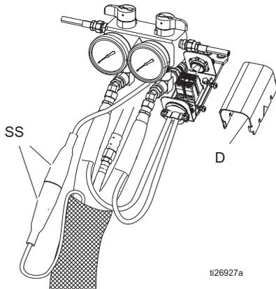
6. Connect cables (SS). Connect electrical connectors (NN). Be sure cables have slack when hose bends. Wrap cable and electrical connections with electrical tape.
