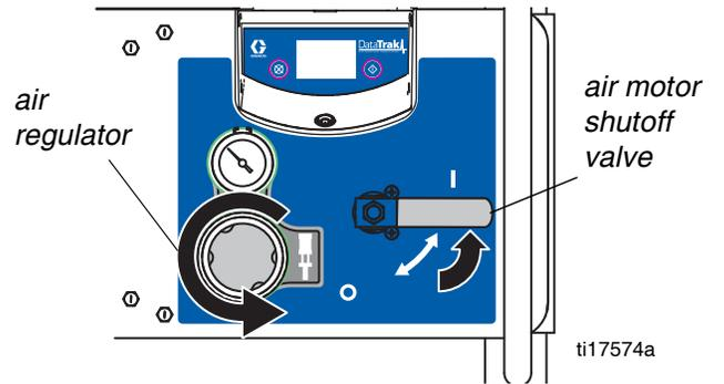
7. Open the air motor shutoff valve.
