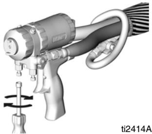
17. Disengage gun piston safety lock.
