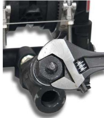
4. Use a wrench to loosen cap fitting located on the front of the Y-strainer.
