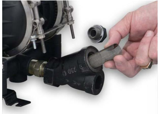
8. Examine screen/filter. If damaged, replace it with new 20 mesh screen, part no.: 129699. Install screen/filter into Y-strainer.
