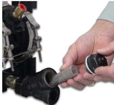
6. Remove screen/filter from Y-strainer.
