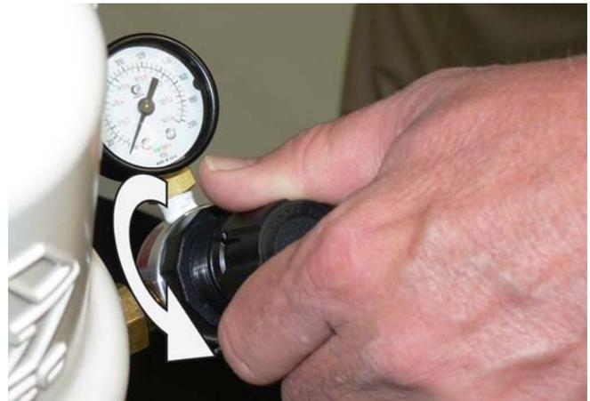
2. Set air regulator pressure to zero psi and/or turn off main air supply.
