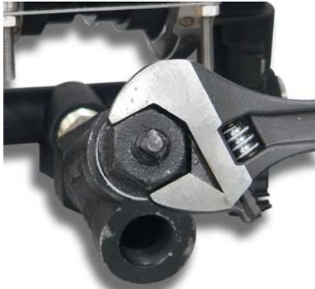
9. Replace and hand tighten fitting in Y-strainer. Use a wrench to tighten securely.
