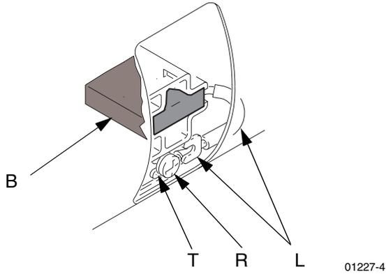
6. Inspect commutator for excessive pitting, burning, or gouging. Black color on commutator is normal. Have commutator resurfaced by qualified motor repair shop if brushes wear too quickly, or replace motor.
