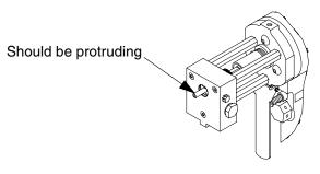
6. Set safety stop to SERVICE (CLOSED), and then pull trigger to determine if weepage occurs in this position.
