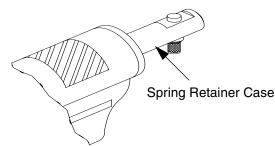
3. Cover open end of air cylinder with hand protected by a cloth and depress gun trigger.
