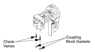
5. Flush open ports and check valves with gun cleaner.
