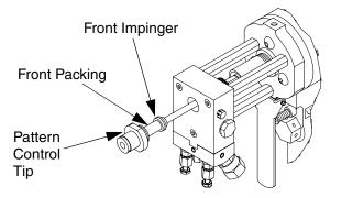
Remove pattern control tip o-ring and front packing from pattern control tip. If packing cannot be removed by hand, use pliers. However, this will require replacement of packings.
