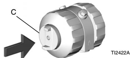
3. Check that o-ring (21) is in position. Liberally lubricate o-ring, threads of lock ring (R) and handle (H), and outside of lock ring. Orient front end (F) as required for desired fluid manifold mounting (bottom mounting is shown).
