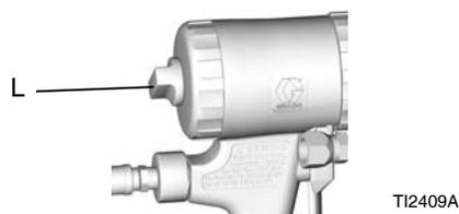
**NOTE:** After the pressure in the spray gun is relieved, the fluid in the hose and proportioner remains under pressure. Follow the **Pressure Relief Procedure** in your proportioner manual to relieve pressure in the system.
