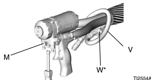
\* Air Valve (W) is not included with spatter pattern spray gun.
