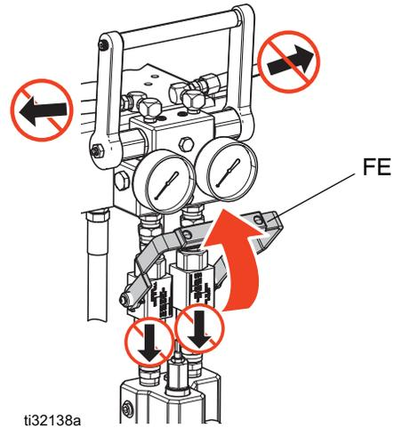
9. Remove pump fluid filters, if installed, and soak in solvent. Clean and replace the filter cap. Always replace the filter o-rings. See your Xtreme pump manual.
