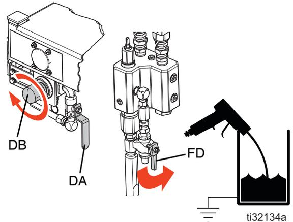
6. Open the solvent flush valve (FD)
