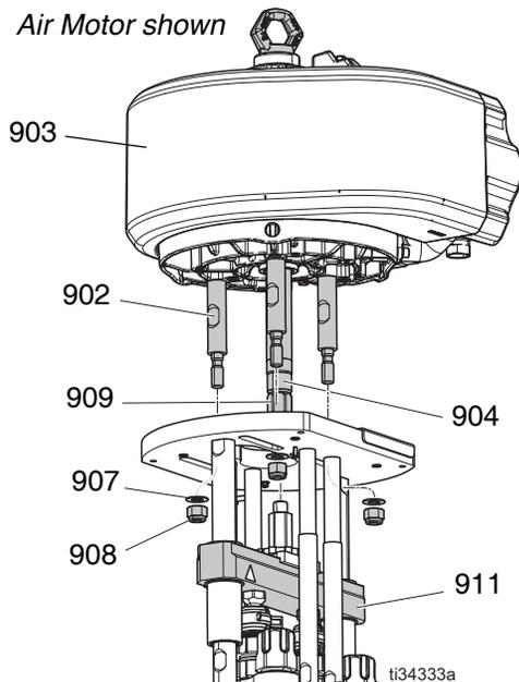
6. Place a wrench on adapter rod (904). Use tool (69) to loosen the serrated yoke nut (909) that holds the air motor (903) above the yoke (911).
