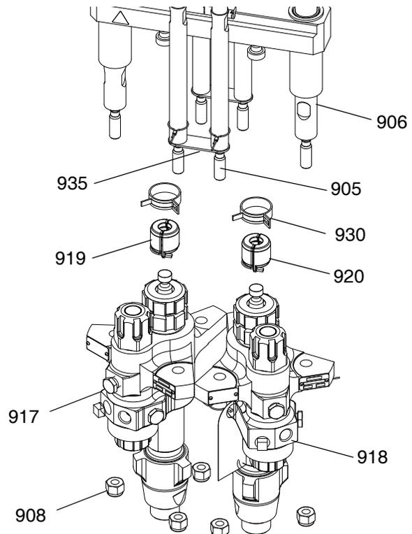
6. Use a wrench to hold the tie rod (905, 906) flats to keep the rods from turning. Unscrew the nuts (908) from the tie rods and carefully remove the displacement pump (917 or 918) and lower straps (935).
