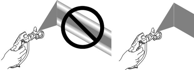
**NOTE:** Excess pressure increases overspray and pump wear.
