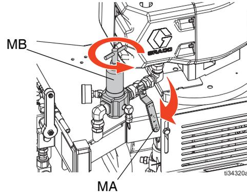
**XP-h Systems only:** Set pump valve on. Then turn down the pressure control knob.
