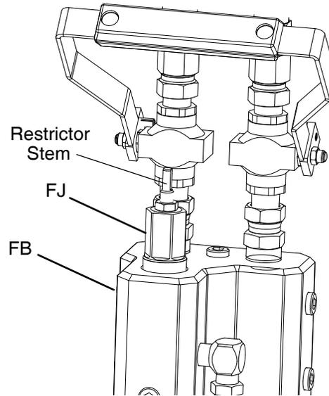
If the mix manifold (FB) is mounted on the machine, you do not need to adjust the restrictor. Leave the restrictor stem open two turns minimum from fully closed.
