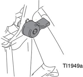
3. **XP Systems:** Turn the main pump air regulator (MB) fully counter-clockwise to shut off.
