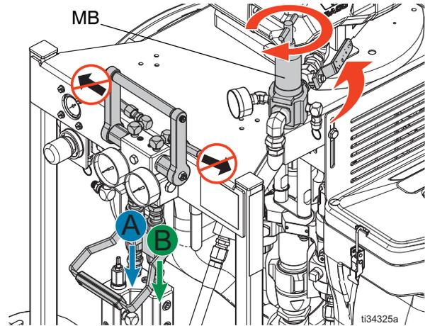
5. Engage the trigger lock and the remove tip. Disengage the trigger lock and trigger the gun while holding against a grounded metal pail. Use a metal pail lid with a hole to dispense through to avoid splashing. Dispense out of the mix hose until a well mixed coating flows from the gun.
