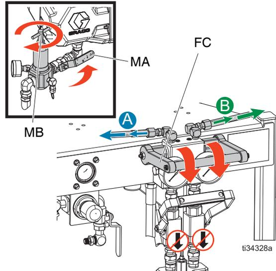
6. Open the motor air shutoff valve (MA).
