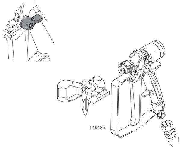
8. Close the solvent pump air valve (DA). Trigger the gun to relieve pressure. Close the solvent flush valve (FD) after relieving the pressure.
