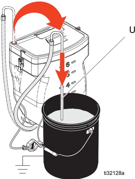
9. Move the recirculation lines (U) back to the correct hopper (J).
