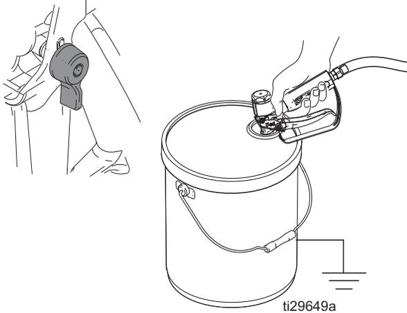
10. Engage the trigger lock. Disassemble and clean the spray tip with solvent by hand. Reinstall on the gun.
