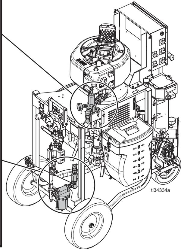
**FIG. 8: Air Control Assembly 26C417**
