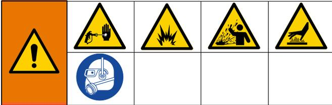
To help prevent injury, wear gloves when using solvents and/or if the fluid temperature exceeds 110 °F (48 °C). To avoid splashing, use the lowest pressure possible to prime.
