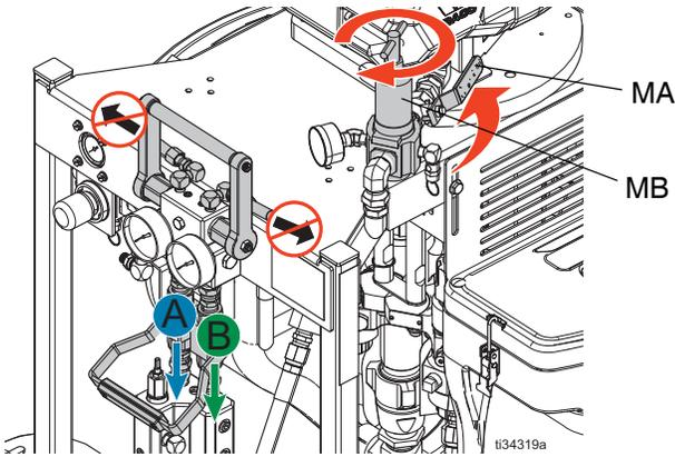
8. Decrease the air regulator pressure (MB). Close the main air shutoff valve (MA).
