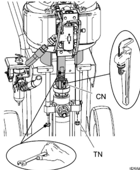
4. Hold the tie rods and remove the tie rod nuts (TN).
