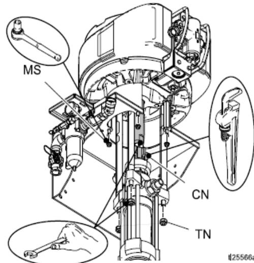
6. Lift up on the air motor to remove it. The tie rods will remain attached.
