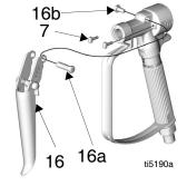
3. Before installing trigger, grease the actuator pins (7) and the pivot pin (16a).
