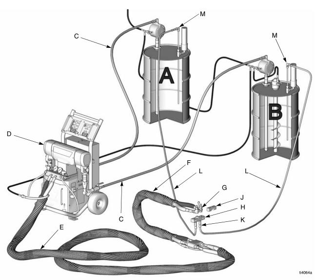
Fig. 1. Circulation System Setup
