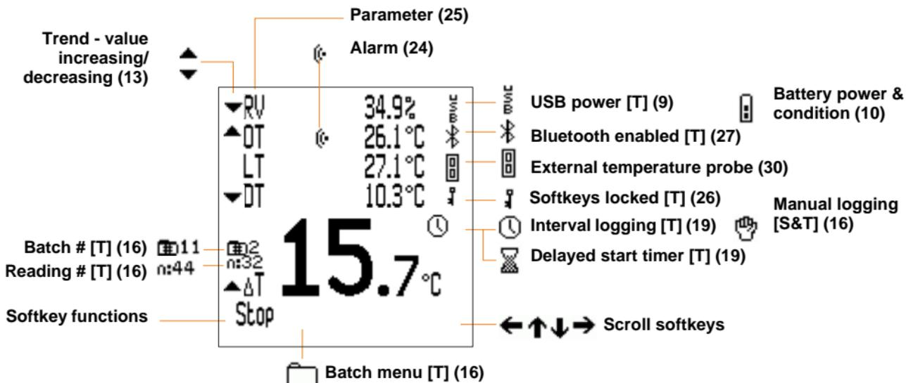
You can select which parameters to show on the reading screen and which of these should be displayed as the Main Reading - see page 28.
