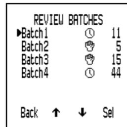
The Review Batch screen is displayed. The screen lists: Batch number, number of readings, date and time batch was created, date and time of last reading, batch type and interval (interval logged batches only).
