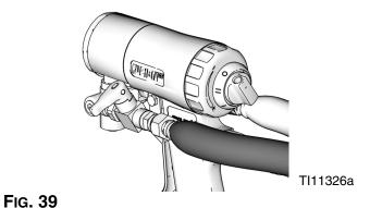
2. Refer to Table 1. Also see identification chart under **Drill Bit Kits**, page 53. Use appropriate size drill bit to clean mix chamber nozzle (N).
