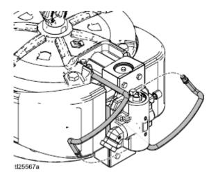
2. Remove four screws (24) and remove the manifold (5) and two gaskets (22). Inspect foam (42) for damage.
