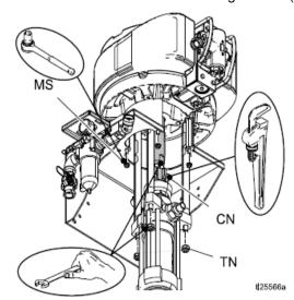
Lift up on the air motor to remove it. The tie rods will remain attached.
