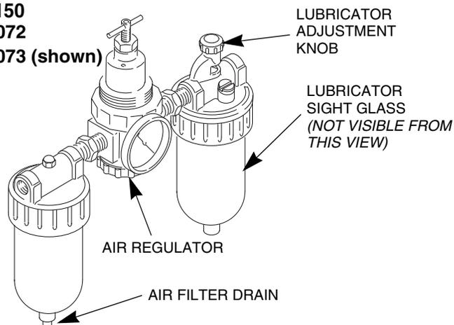
Before installing any air line components, blow out the pipe line to remove scale and other debris. Use pipe compound or tape sparingly and only on male threads.
