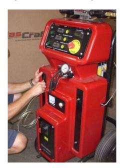
**42.** Hand tighten the screws on the left side.
