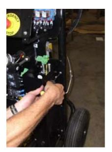
**8.** Use a 5/32 in. hex key wrench and remove the 5 screws from the front heater support bracket.
