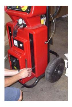
**43.** Use a 5/16 in. wrench and tighten all 4 screws.
