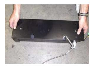
**24.** • Place the heater support bracket on the replacement heater.
