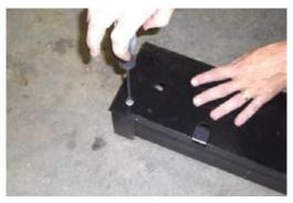
**17.** Use a 5/32 in. hex key wrench to remove the bottom screw.
