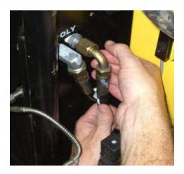
**34.** Hand tighten the inlet hose fitting.
