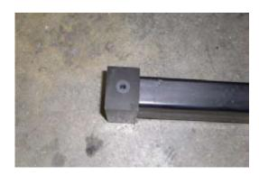
**23.** Place the bottom support washer over the screw hole.
