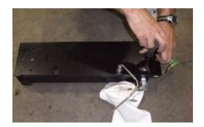
**18.** Use a 5/32 in. hex key wrench to remove the top screw.
