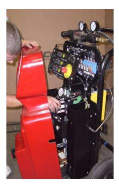
**39.** The "red" cover can be reattached to the system (not shown above) slide the cover back up the heated hose, lift and grab the wires to help in placement.
