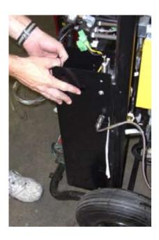
**28.** Align the heater support bracket with the holes and replace the 5 screws, tighten securely.
