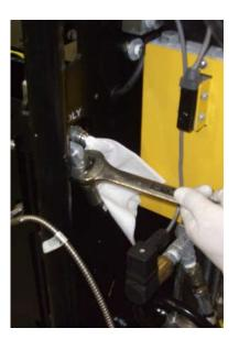
**14.** Use a 5/16 in. wrench to loosen the fitting on the outlet hose. Use a clean up towel to catch any spillage and carefully stretch out the outlet hose.
