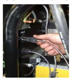
**38.** Carefully connect the thermocouple plug into the receptacle.
