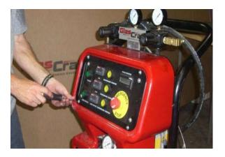
**45.** Use a 5/16 in. hex key wrench and tighten all 4 screws.
