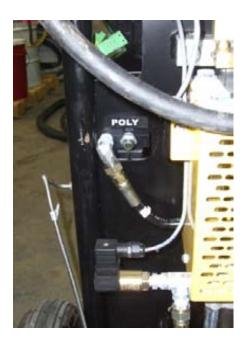
**32.** Tighten the outlet hose fitting by hand.
