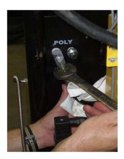
**33.** Use a 15/16 in. wrench and tighten the outlet hose fitting tight.
