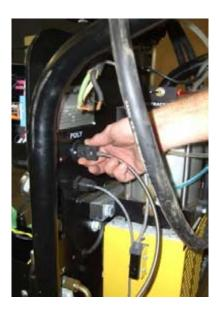
**10.** At the back of the system carefully unplug the thermocouple connector.
