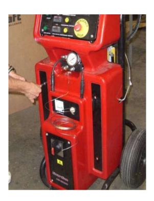
**4.** Use a 5/16 in. wrench and remove the screws from the left side.
