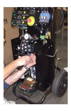
**30.** Use a 5/32 in. hex key wrench and tighten the 5 screws securely
