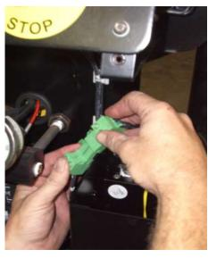
**37.** Carefully reconnect the large green connector by aligning the two ends and pushing them together.
