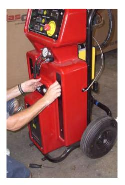
**41.** Hand tighten the screws on the right side.
