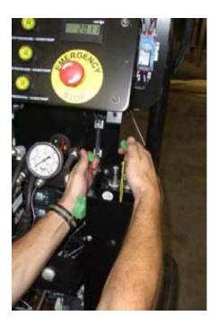
**7.** Carefully disconnect the small green connector by pulling it apart.
