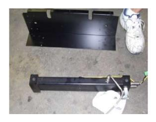
**19.** Separate the heater support bracket from the heater.
