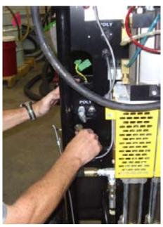
**31.** Atach the outlet hose to the elbow fitting
