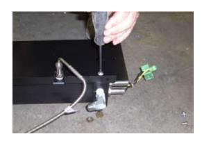
**26.** Reinstall the top screw to the heater and tighten.
