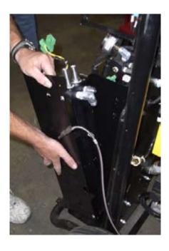
**27.** Install the new heater and support bracket back onto the system.
