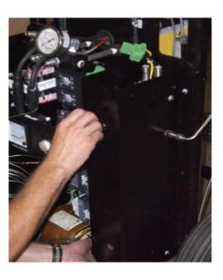
**29.** Align the front heater support bracket to the heater support bracket and hand tighten the 5 screws.
