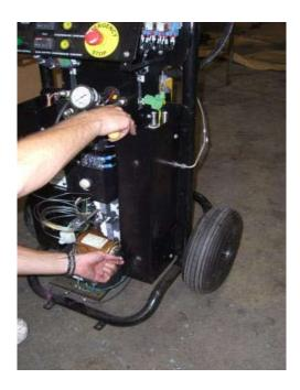
**9.** Remove the heater support bracket and set it to the side, to be reused.
