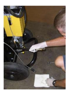
**12.** Carefully stretch the inlet hose out, use a clean up towel to stop any spillage of material.
