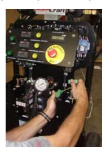
**6.** Complete the POLY side first (steps 6 - 38). Carefully disconnect the large green connector by pulling it apart. Replace the POLY side first before starting the ISO side.
