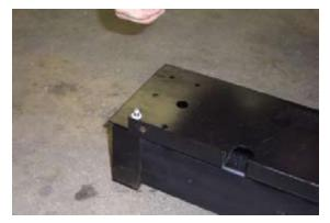
**25.** Reinstall the bottom screw to the heater and tighten.
