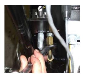
**35.** Use a 7/8 in. wrench and tighten the inlet hose fitting tight.
