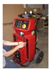
**3.** Use a 5/16 in. wrench and remove the 4 screws in the top trim ring.
