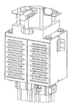
**15.** Assemble the bottle bracket GC1840 (included with kit) to the fluid section. The bottle bracket can be attached to either side of the air motor or either side of the pump plate as shown.
