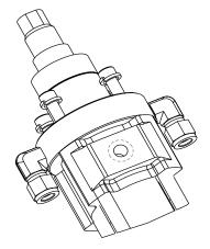
13. Reattach the ISO pump to the pump plate. Attach the pump shaft extension to the pump saddle ONE and TWO. Tighten the pump to the plate using the new mounting bolts and lock washers provided with the kit (this will allow for proper alignment).
