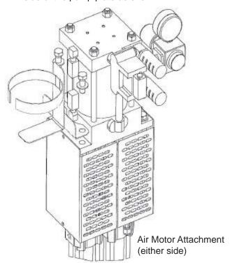
Mount the bottle bracket to the top for hydraulic units.
