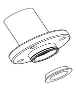
b. Remove the seal. Save or discard the solvent cup and o-ring.
