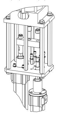
**6.** Remove the ISO pump shaft extension.
