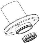
**10.** Install the seal and support washer to the new solvent cup adapter assembly included with the kit.
