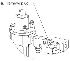
b. Remove Switch from fitting.
