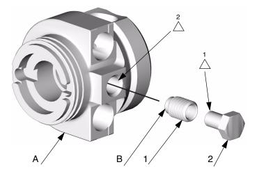
Apply lubricant to end of bolt (2).
