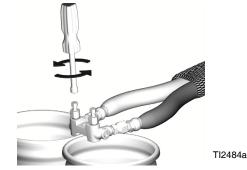
FIG. 21: Open Manual Valves
