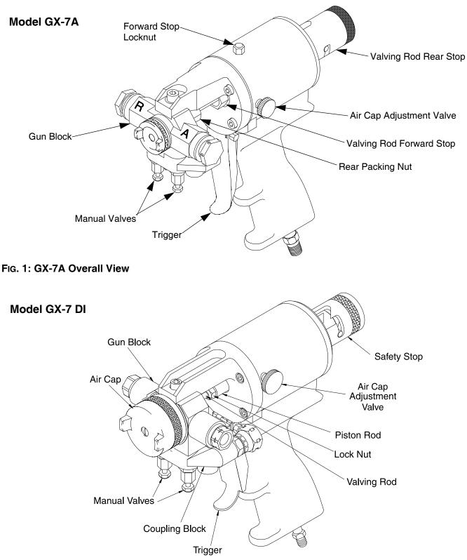
FIG. 2: GX-7 DI Overall View
