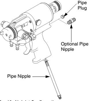
FIG. 16: Air Inlet Configuration
