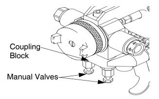
FIG. 14: Open Manual Valves
