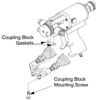
FIG. 15: Install Coupling Block
