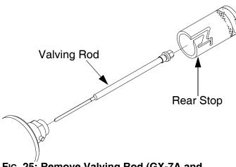
FIG. 25: Remove Valving Rod (GX-7A and GX-7 400 models)
