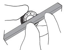
FIG. 28: Unthread Cap from PCD Body
