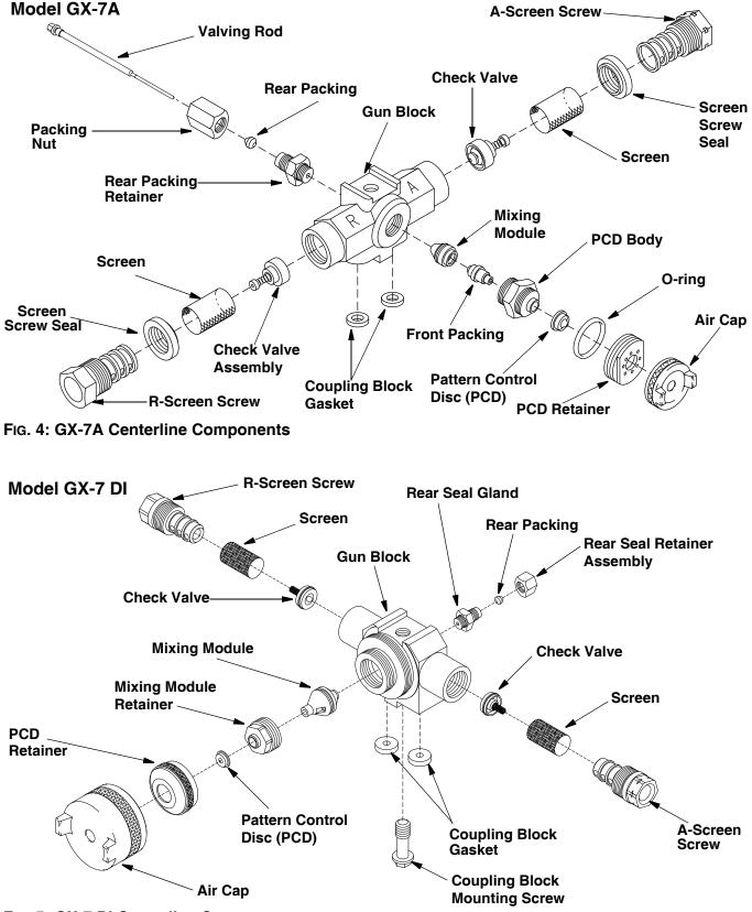
FIG. 5: GX-7 DI Centerline Components
