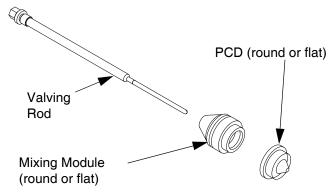
FIG. 7: GX-7A Mixing Module
