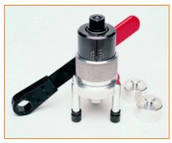
Elcometer 106/6 Coatings on Concrete Adhesion Tester
