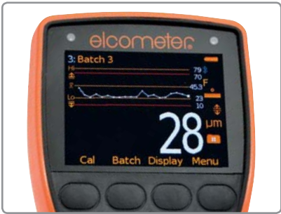
On-screen trend graph displaying last 20 measurement values
