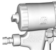
3. Close gun fluid inlet valves A and B.
