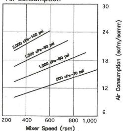
Choose mixer speed across bottom of chart and follow up to material viscosity. Approximate required air flow is shown at right. Required air pressure is shown beside viscosity, but will vary with material.
