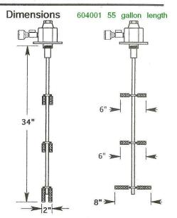
Ar rest, blades will fit through a 2" bung opening. While spinning, blades extend to the diameters shown.
